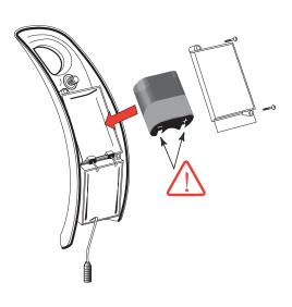
4. Insert a new 6 Volt Type 2CR5 Lithium Battery. The red LED will flash for one (1) minute. Reinstall Battery Cover. Reconnect electrical lead at connector if previously disconnected. Reinstall Throat Plate. If LED doesn't flash or if it just lights up, remove and then reinsert the Battery. If water flows continuously after inserting the new Battery and opening the Supply Stops, remove and then reinsert the Battery.
